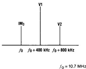
FIGURE 13. Spectrum Analyzer Display of Tuner Output
