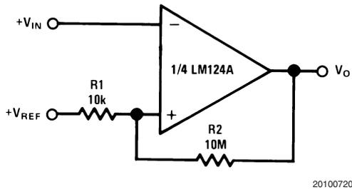
Ground Referencing a Differential Input Signal
