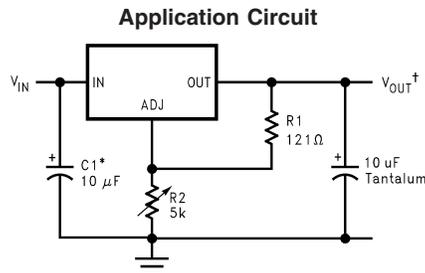
\*NEEDED IF DEVICE IS FAR FROM FILTER CAPACITORS
