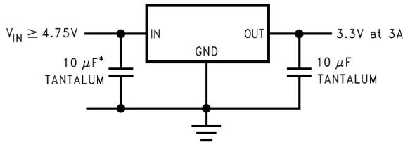
\*MAY BE OMITTED IF INPUT SUPPLY IS WELL BYPASSED WITHIN 2" OF THE LM1085
