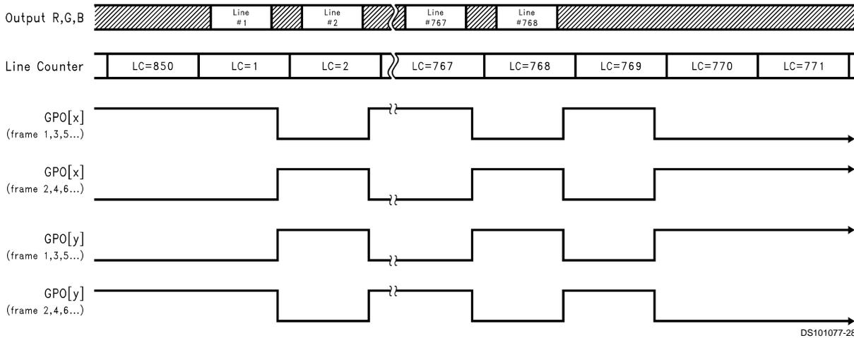
FIGURE 25. Example #4c: GPO Vertical Scope View
