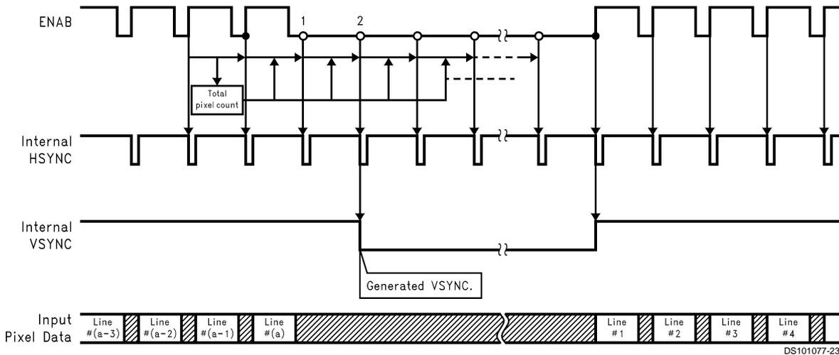
**FIGURE 20. ENAB ONLY MODE and Internally Generated Timing**
