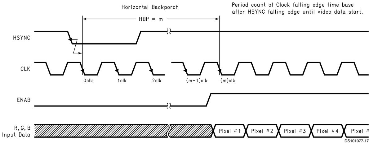
Note: Horizontal Position determined by ENAB if FIX\_VERT = "0" and ENAB is active.
