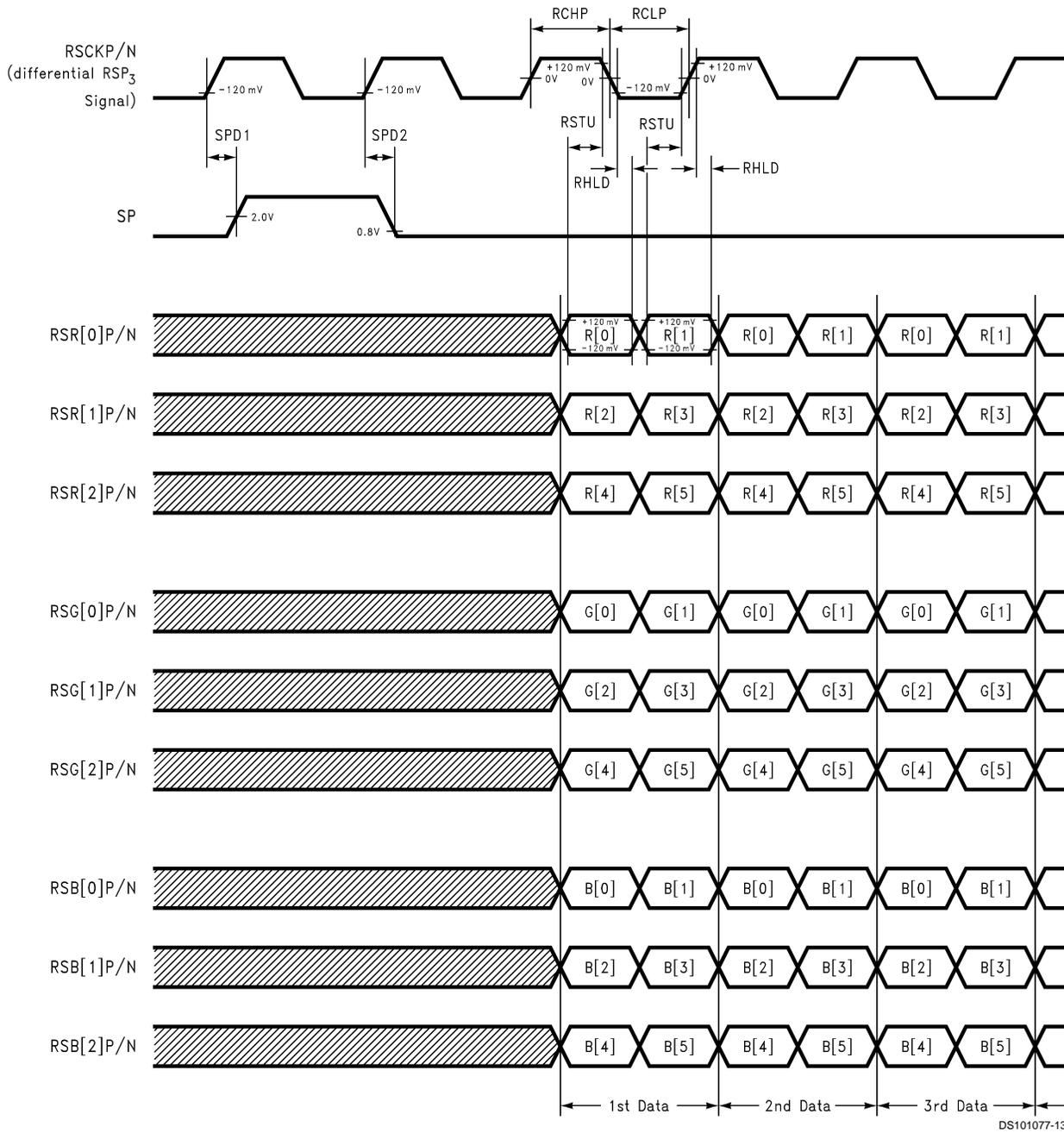
Note: RSCP/N, RSR[2:0]P/N, RSG[2:0]P/N and RSB[2:0]P/N are differential outputs, SP is single ended output.
