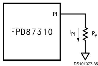
FIGURE 13. R<sub>PI</sub> Connection Diagram
