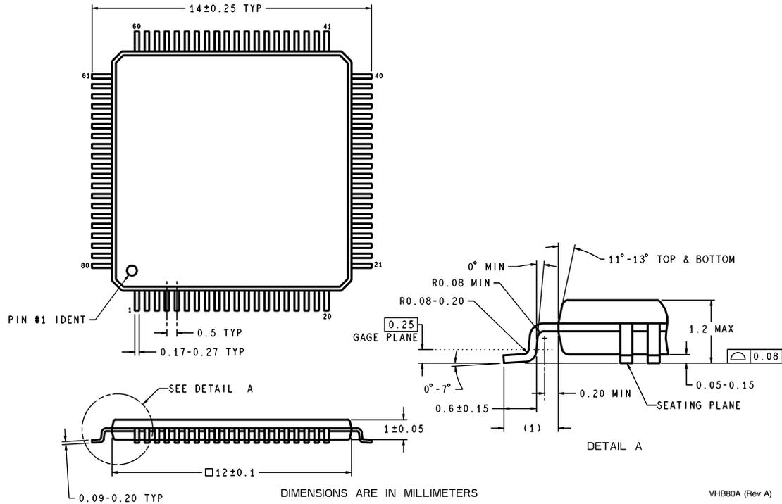
**Thin Plastic Quad Flatpak (TQFP)**
