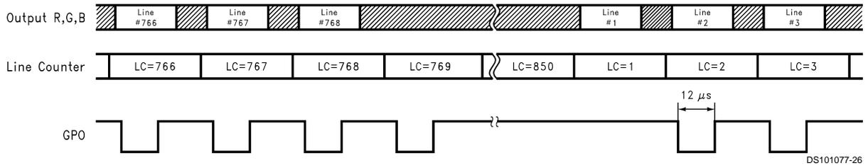
FIGURE 23. Example #4b: GPO Vertical Scope View
