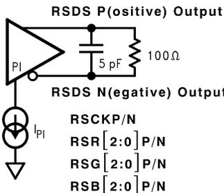
$$V_{RSCK} = V_{RSCKP} - V_{RSCKN}$$
