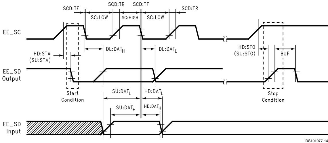
FIGURE 9. EEPROM Interface Bus Timing
