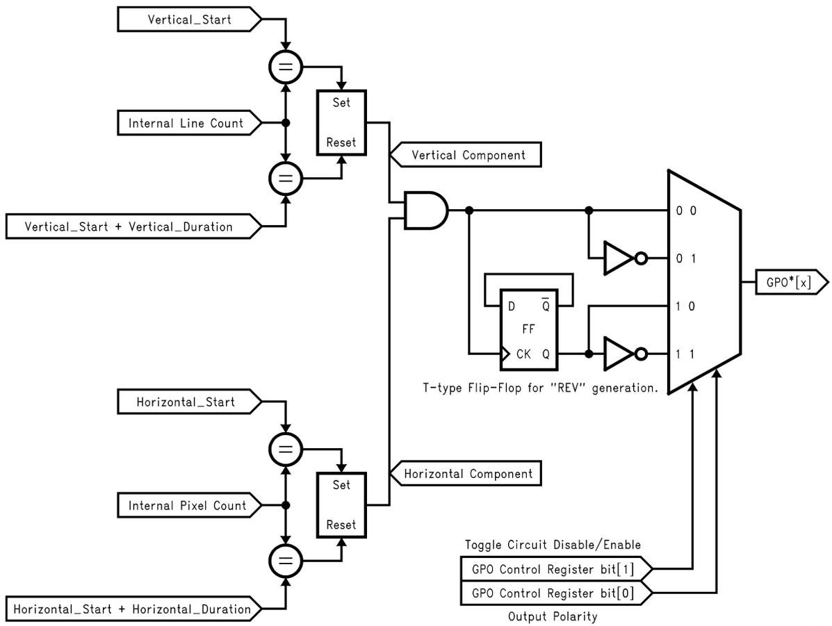
FIGURE 27. GPO (General Purpose Output) Generation Method
