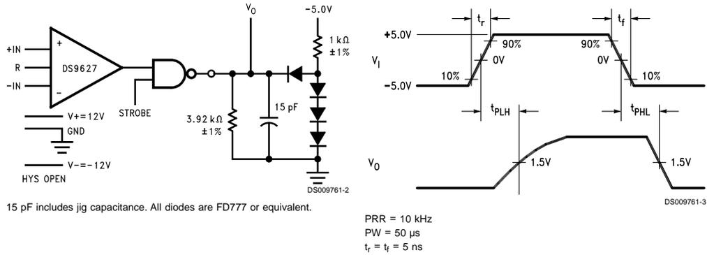
FIGURE 1. Switching Time Test Circuit and Waveforms
