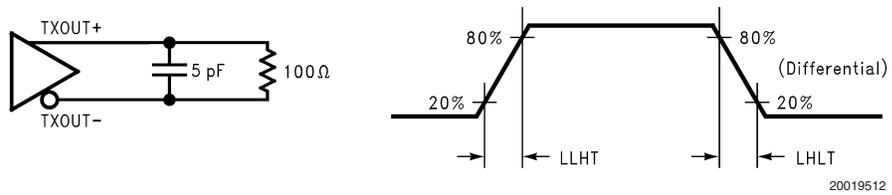
**FIGURE 2. LVDS Output Load and Transition Times**
