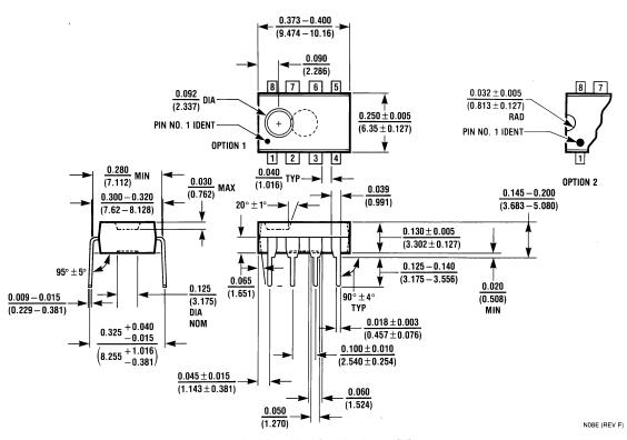
Molded Dual-In-Line Package (N) Order Number DS8921N, DS8921AN or DS8921ATN **NS Package Number N08E**
