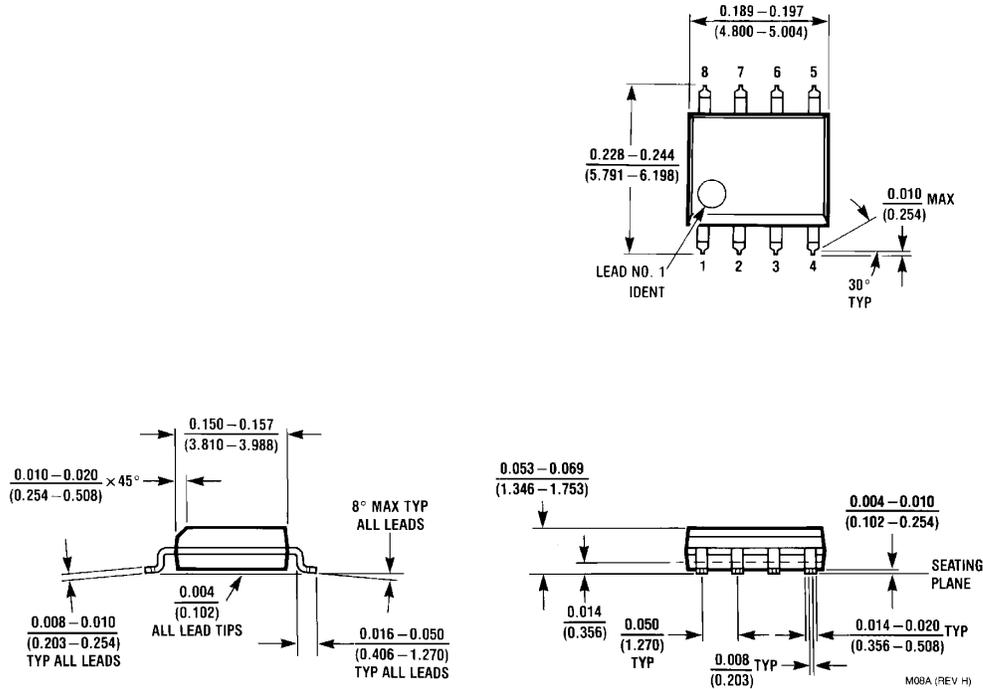
**Molded SOIC Package (M)**
