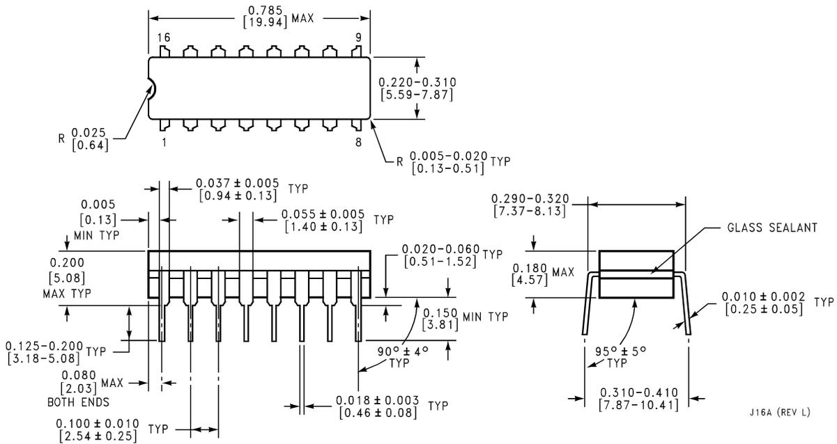
**16 Lead Ceramic Dual-in-Line Package (J)**
