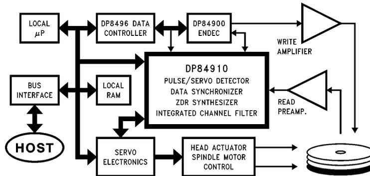
FIGURE 1. DP84910 in a Typical Disk Drive System
