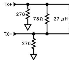
**Note:** In the above diagram, the TX+ and TX- signals are taken from the AUI side of the isolation (pulse transformer). The pulse transformer used for all testing is the Pulse Engineering PE64103.
