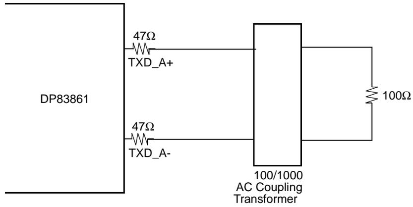
Figure 18. 100 Mb/s Twisted Pair Load (zero meters)
