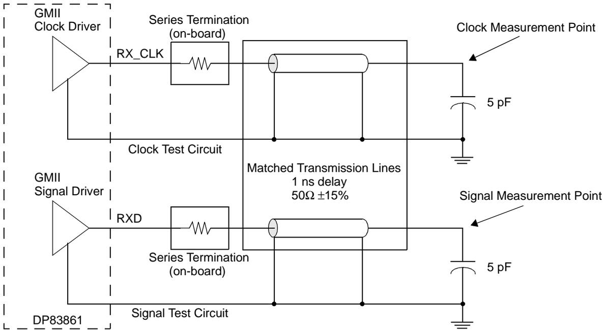
Figure 22. GMII Setup and Hold Time Test Circuit
