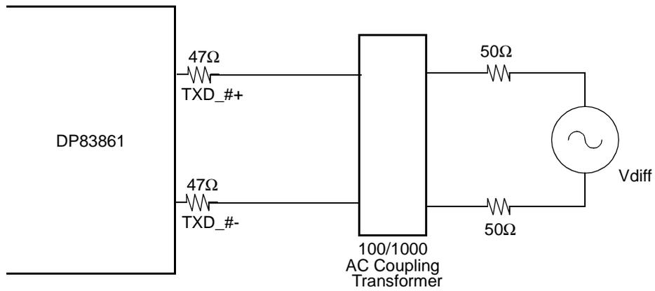
Figure 19. 1000 Mb/s Twisted Pair Load (zero meters)
