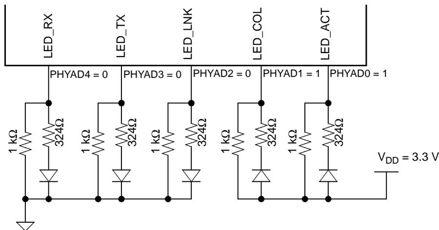
**Figure 5. PHYAD Strapping and LED Loading Example**
