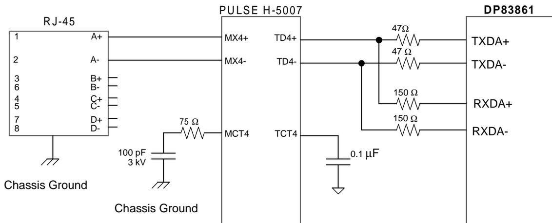
Only the connections for one of the twisted pair channels is shown. Connections for channels B, C, D are similar.
