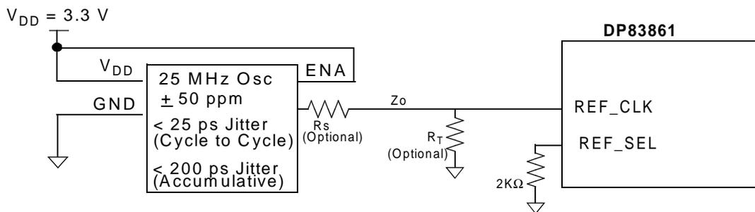
Figure 4. 25 MHz Oscillator Option
