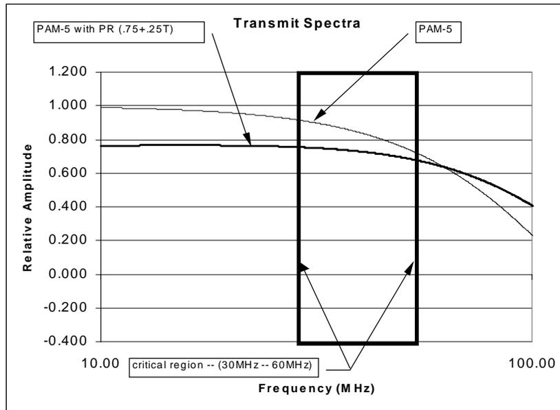
Figure 9. Effect on Spectrum of PR-shaped PAM-5 coding
