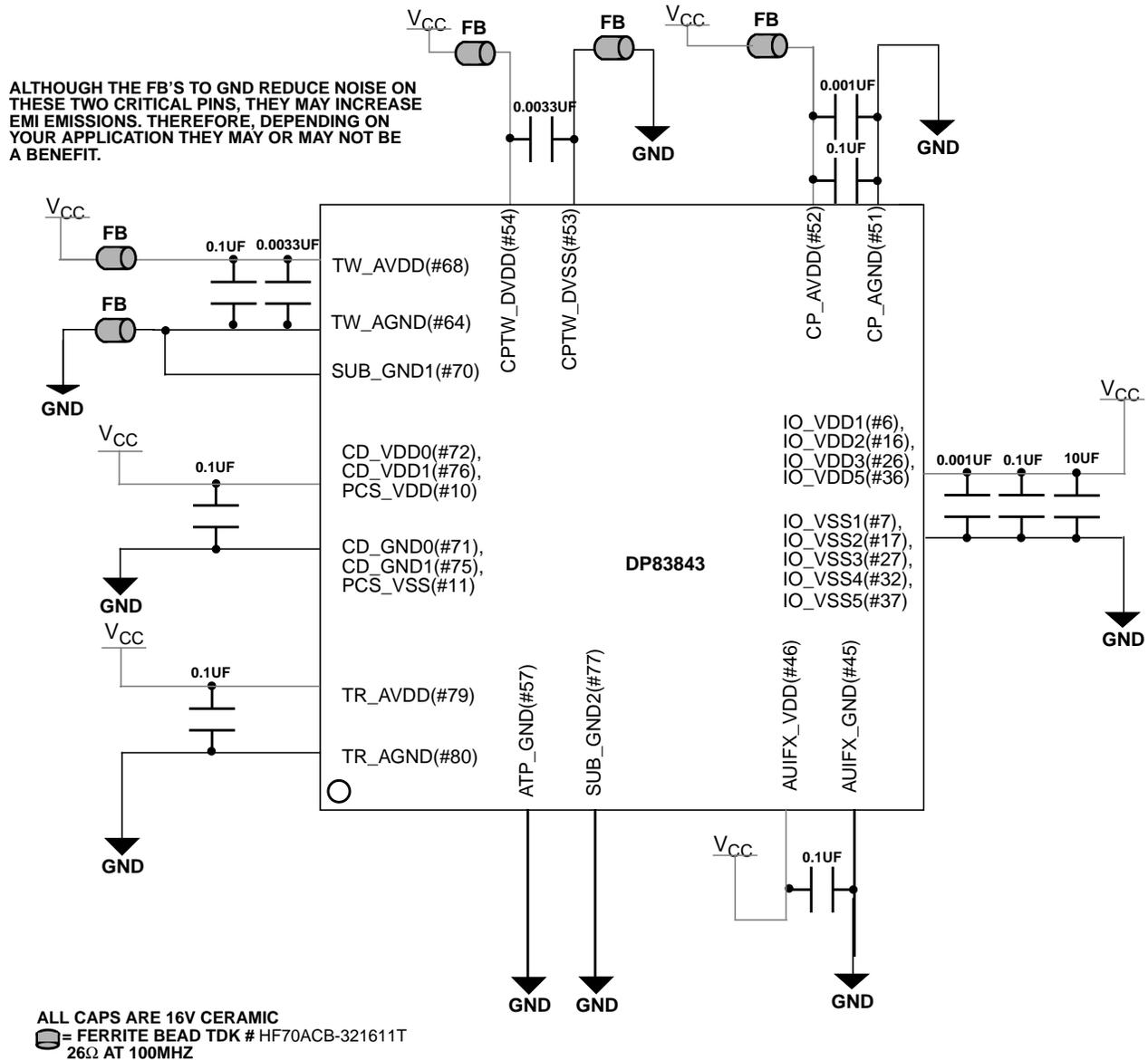
Figure 23. Power and Ground Filtering for the DP83843
