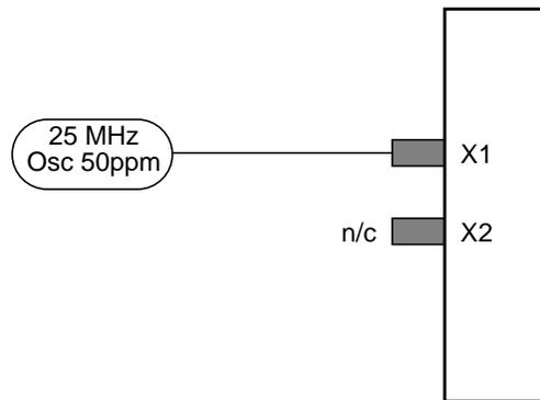
Figure 20. Oscillator Reference Clock Connection Diagram
