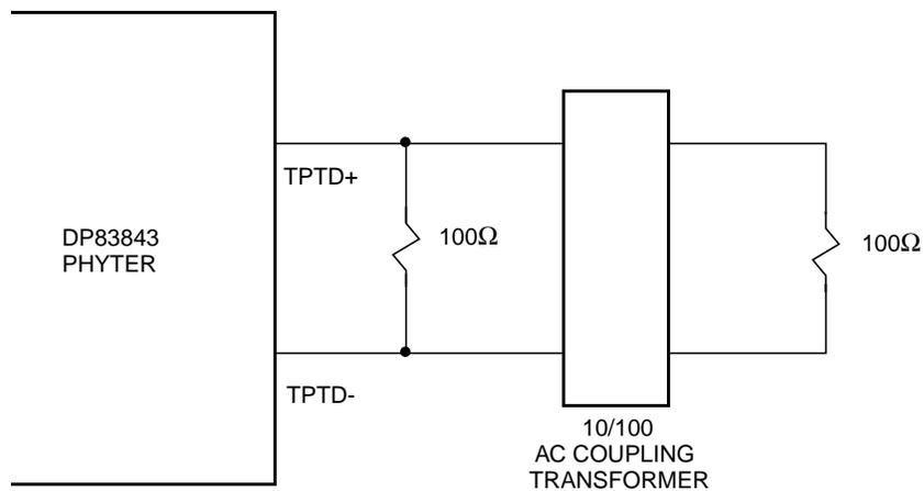
**Figure 29. 10/100 Twisted Pair Load (zero meters)**
