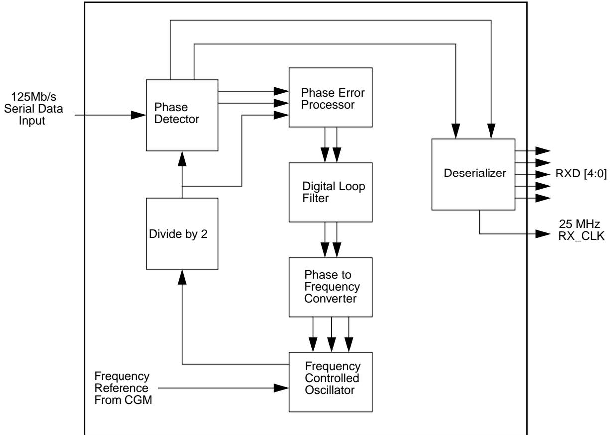
Figure 18. 100BASE-X Clock Recovery Module block diagram
