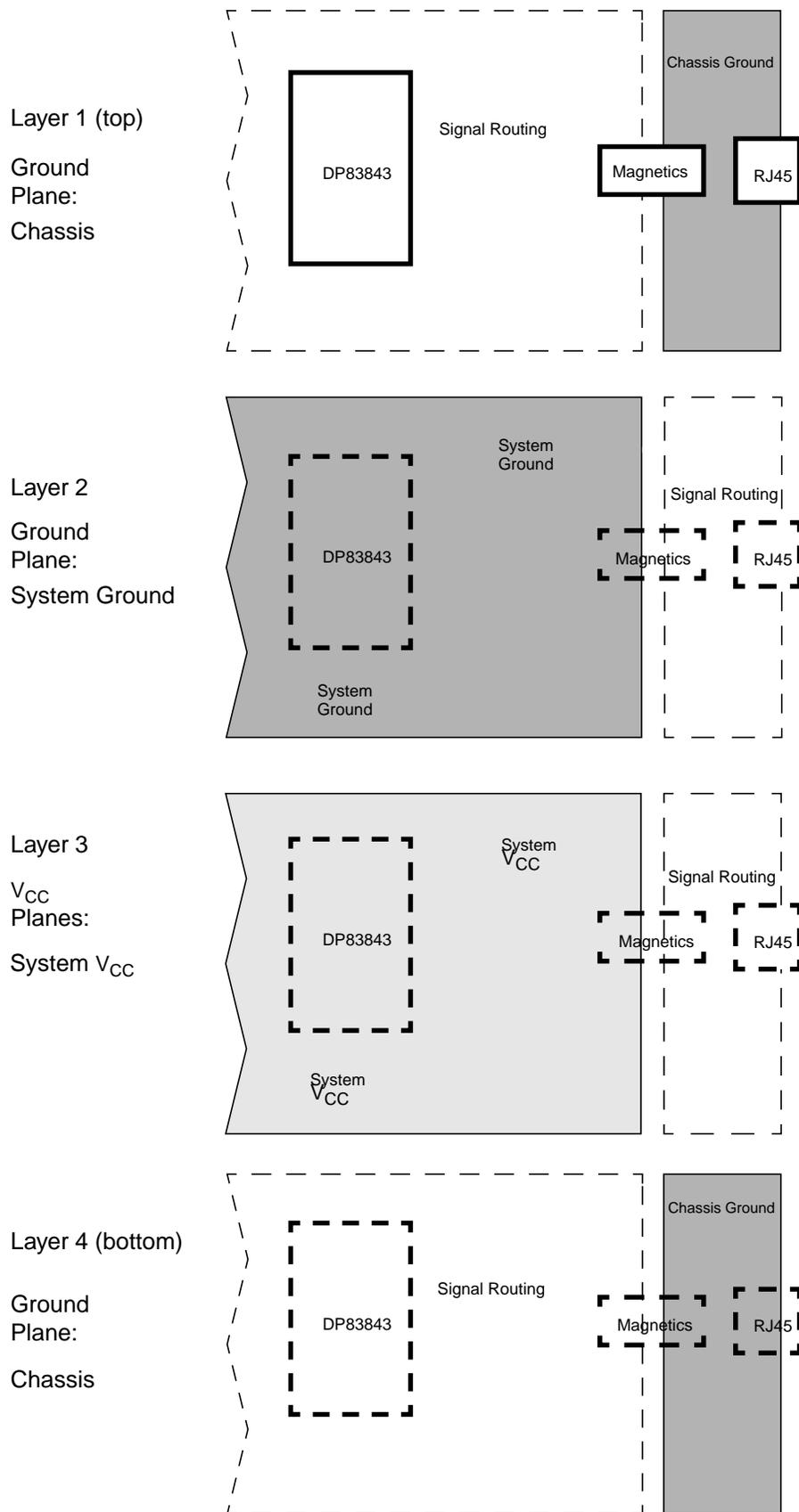
Figure 24. Typical plane layout recommendation for DP83843
