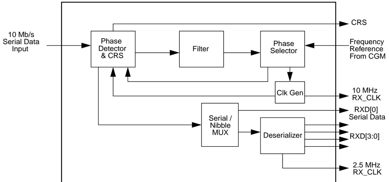
Figure 19. 10M Manchester Clock Recovery Module block diagram
