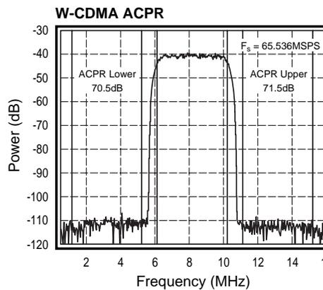
**DAC14135 Typical Performance Characteristics** ( $A_{V_{DD}} = +5V$ ,  $DV_{DD} = +5V$ ,  $CV_{DD} = +5V$ ,  $T_A = 25^\circ C$ )
