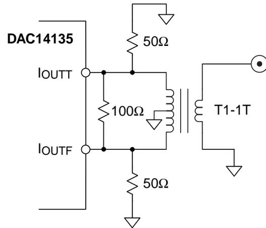
**Figure 4: AC Coupled Differential to Single-ended Topology**
