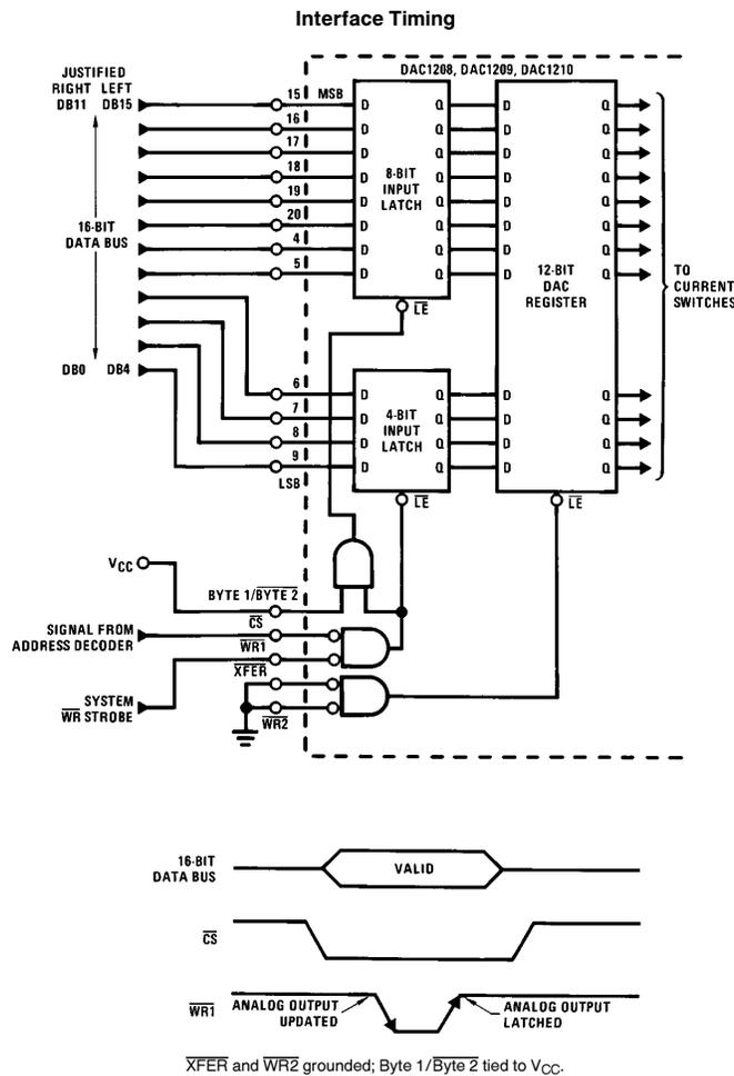
XFER and WR2 grounded; Byte 1/Byte 2 tied to VCC.
