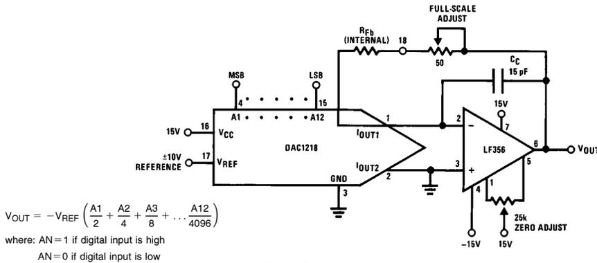
FIGURE 2. Unipolar Output Voltage
