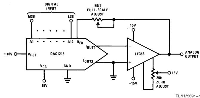
$$V_{OUT} = -V_{REF} \left( \frac{A1}{2} + \frac{A2}{4} + \frac{A3}{8} + \dots + \frac{A12}{4096} \right)$$
