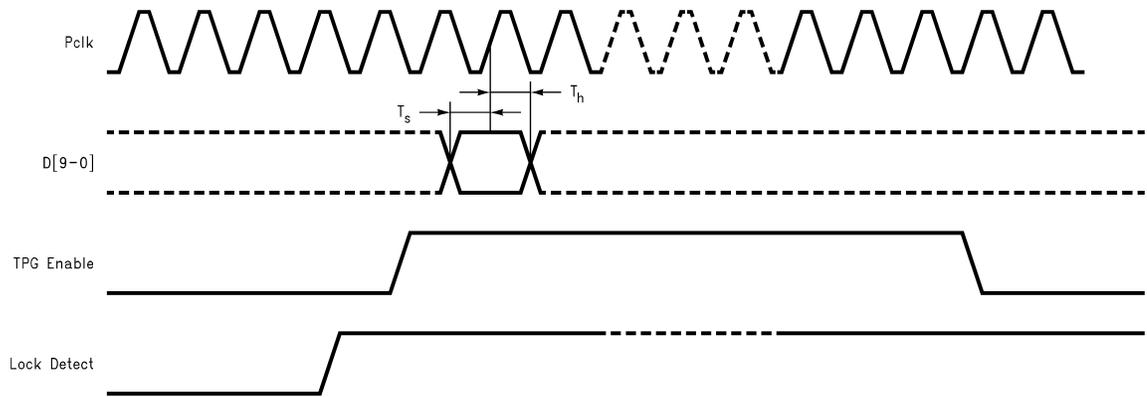
FIGURE 3. Setup and Hold Timing
