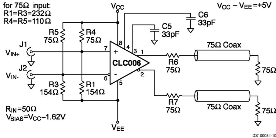
FIGURE 7. Differential Input DC Coupled Output
