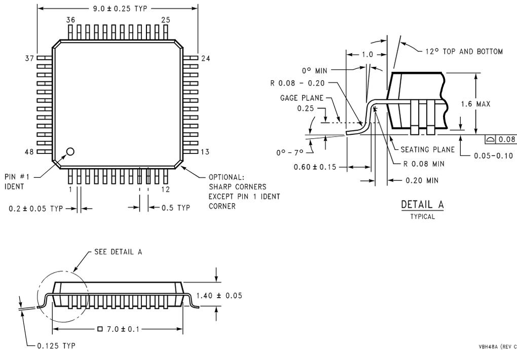
**48-Lead TQFP Package**
