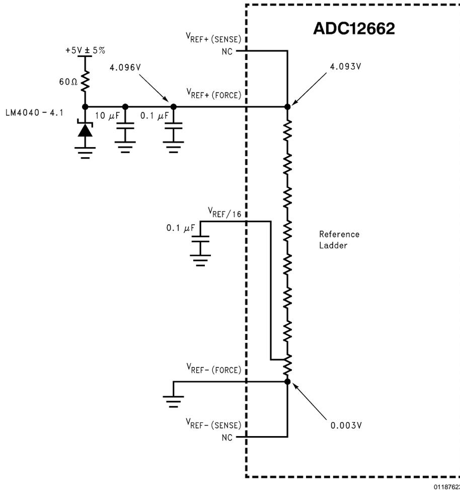
FIGURE 11. Using the  $V_{REF}$  Force Pins Only**5.0 POWER SUPPLY CONSIDERATIONS**
