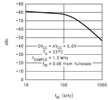
**SINAD vs Input Frequency (Through Mux)**
