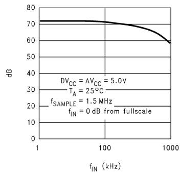
**THD vs Input Frequency (Through Mux)**
