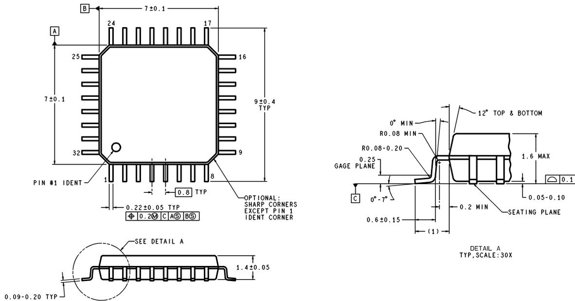
DIMENSIONS ARE IN MILLIMETERS
