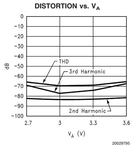
**Typical Performance Characteristics**  $V_A = V_D = 3.3V$ ,  $V_{DR} = 2.5V$ ,  $f_{CLK} = 40\text{ MHz}$ ,  $f_{IN} = 10.4\text{ MHz}$ , unless otherwise specified (Continued)
