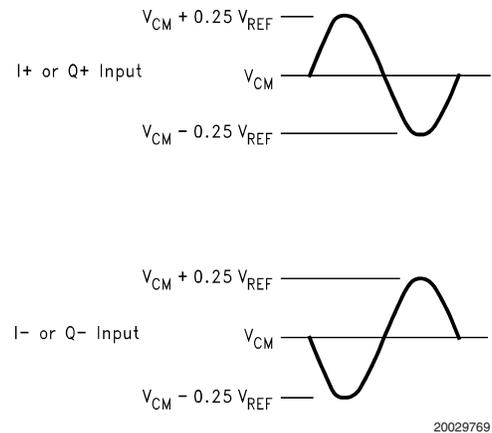
**FIGURE 2. The ADC10D040 is designed for use with differential signals of  $1.4 V_{P-P}$  with a common mode voltage of 1.5V. The signal swing should not cause any pin to experience a swing more than 300 mV beyond the supply rails.**
