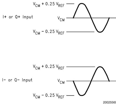
**FIGURE 2. The ADC10D020 is designed for use with differential signals of 1.0 V<sub>P-P</sub> with a common mode voltage of 1.5V. The signal swing should not cause any pin to experience a swing more than 300 mV beyond the supply rails.**
