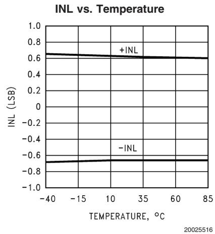
**Typical Performance Characteristics**  $V_A = V_D = V_{DR} = 3.0V$ ,  $f_{CLK} = 20$  MHz, unless otherwise specified (Continued)
