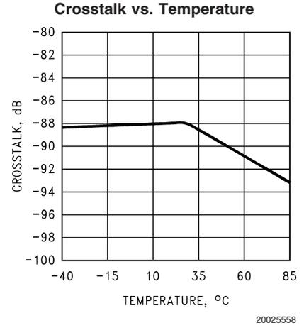
**Typical Performance Characteristics**  $V_A = V_D = V_{DR} = 3.0V$ ,  $f_{CLK} = 20\text{ MHz}$ , unless otherwise specified (Continued)
