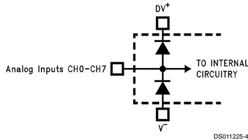
**Note 9:** A diode exists between  $AV^+$  and  $DV^+$  as shown below.
