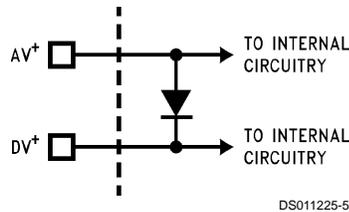
To guarantee accuracy, it is required that the  $AV^+$  and  $DV^+$  be connected together to a power supply with separate bypass filter at each  $V^+$  pin.
