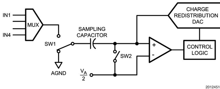
FIGURE 2. ADC084S021 in Hold Mode
