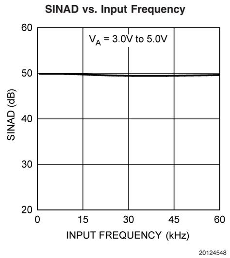
**Typical Performance Characteristics**  $T_A = +25^{\circ}\text{C}$ ,  $f_{\text{SAMPLE}} = 50 \text{ kSPS to } 200 \text{ kSPS}$ ,
