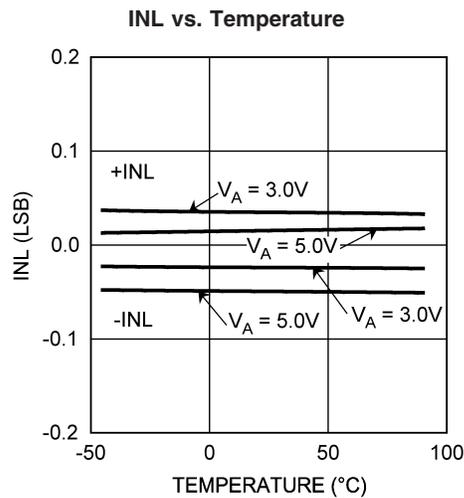
**Typical Performance Characteristics**  $T_A = +25^\circ\text{C}$ ,  $f_{\text{SAMPLE}} = 50 \text{ kSPS to } 200 \text{ kSPS}$ ,
