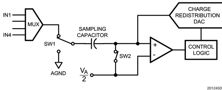
FIGURE 1. ADC084S021 in Track Mode
