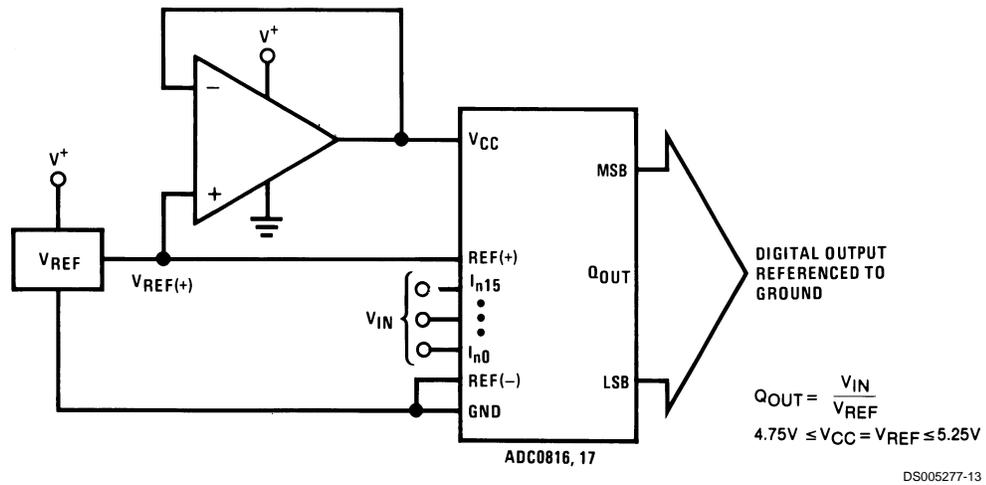
FIGURE 11. Ground Referenced Conversion System with Reference Generating V<sub>CC</sub> Supply
