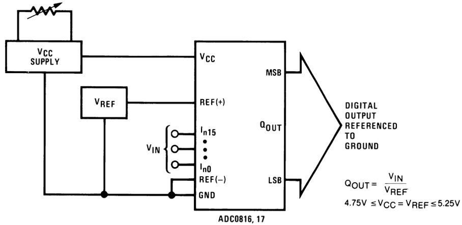
FIGURE 10. Ground Referenced Conversion System Using Trimmed Supply
