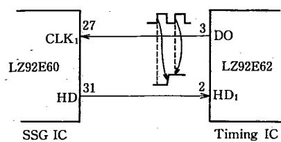
One cycle of DO output is 104ns for a 512-pixel (H) CCD, and 79ns for a 760-pixel (H) CCD.
