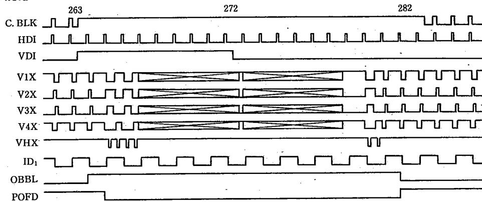
(3) NTSC vertical timing 3 (Electronic shutter speed : 1/2000 sec)
