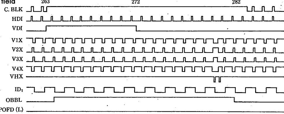
**(2) NTSC vertical timing 2 (Electronic shutter speed : 1/1000 sec)****Odd field**
