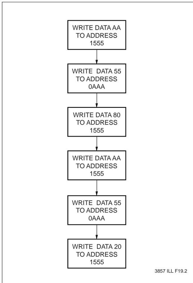
In the event the user wants to deactivate the software data protection feature for testing or reprogramming in an E<sup>2</sup>PROM programmer, the following six step algorithm will reset the internal protection circuit. After  $t_{WC}$ , the X28HC64 will be in standard operating mode.
