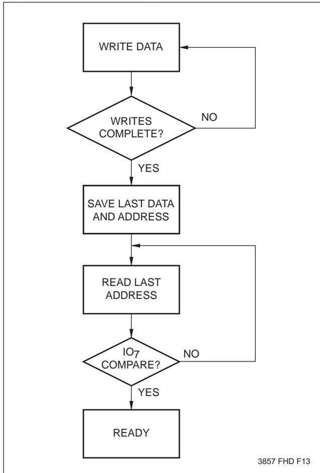
DATA Polling can effectively reduce the time for writing to the X28HC64. The timing diagram in Figure 2 illustrates the sequence of events on the bus. The software flow diagram in Figure 3 illustrates one method of implementing the routine.
