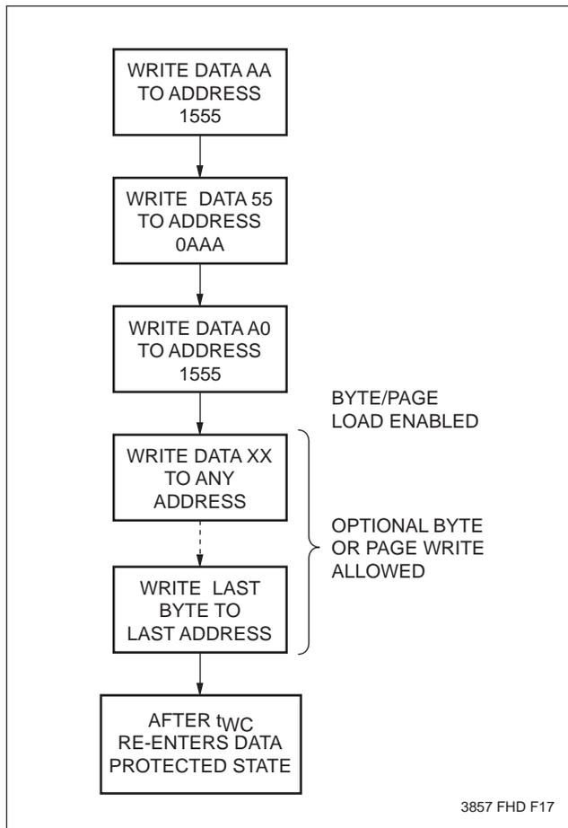
Regardless of whether the device has previously been protected or not, once the software data protection algorithm is used, the X28HC64 will automatically disable further writes unless another command is issued to deactivate it. If no further commands are issued the X28HC64 will be write protected during power-down and after any subsequent power-up.
