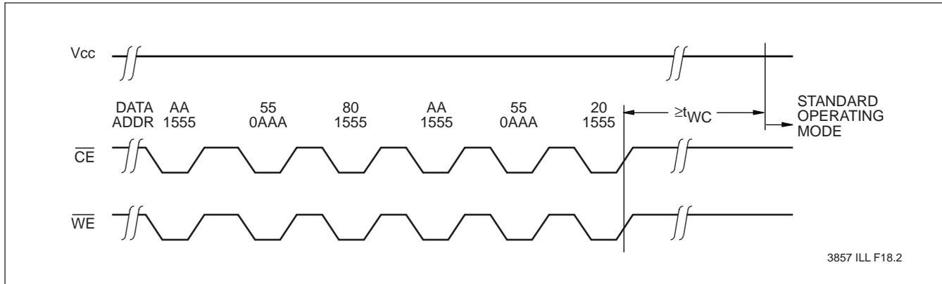
Figure 9. Software Sequence to Deactivate Software Data Protection
