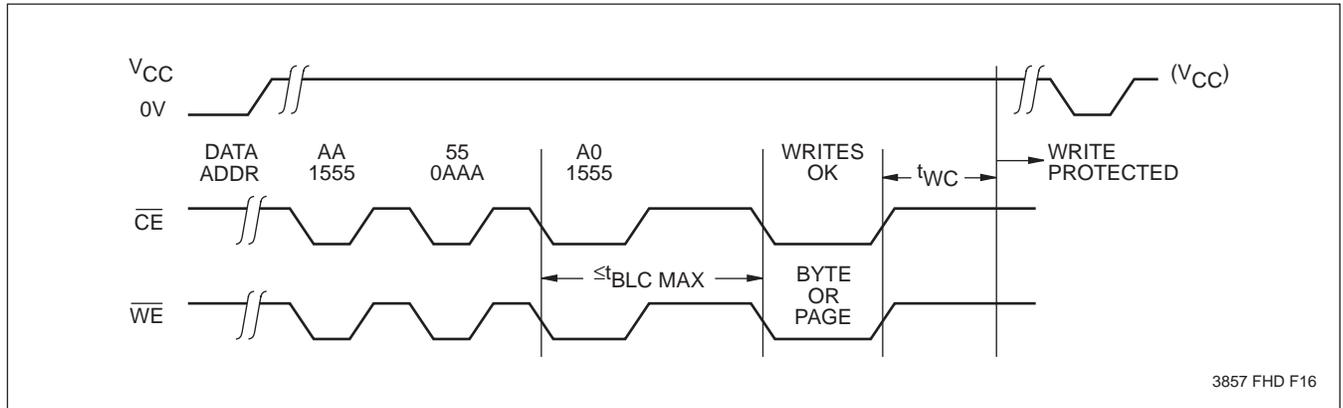
Figure 7. Write Sequence for Software Data Protection
