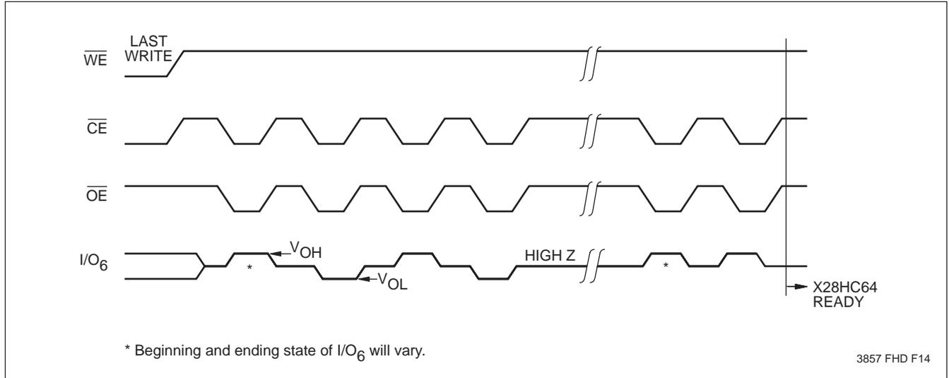
Figure 5. Toggle Bit Software Flow
