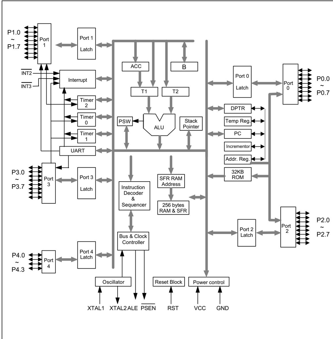
Figure 2. Architecture of the W78C58
