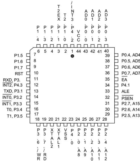
44-Pin QFP/TQFP (W78C58F/W78C58M)
