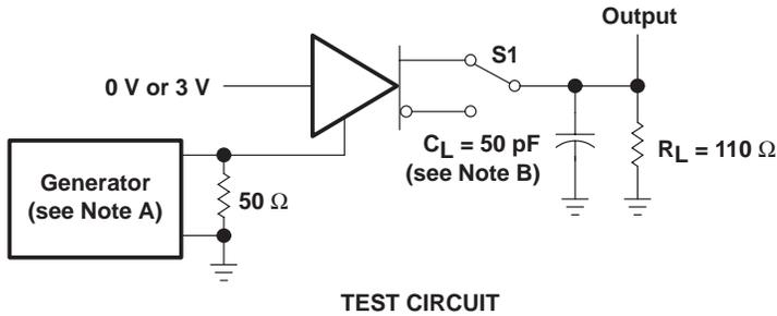
NOTES: A. The input pulse is supplied by a generator having the following characteristics: PRR  $\leq$  1 MHz, 50% duty cycle,  $t_r \leq 6$  ns,  $t_f \leq 6$  ns,  $Z_O = 50 \Omega$ .
