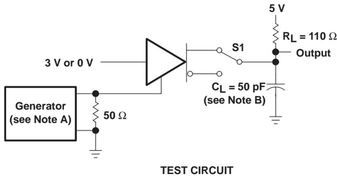
NOTES: A. The input pulse is supplied by a generator having the following characteristics: PRR  $\leq$  1 MHz, 50% duty cycle,  $t_r \leq 6$  ns,  $t_f \leq 6$  ns,  $Z_O = 50 \Omega$ .
