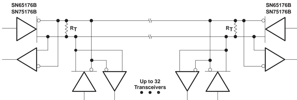
NOTES: A. The line should be terminated at both ends in its characteristic impedance ( $R_T = Z_0$ ). Stub lengths off the main line should be kept as short as possible.
