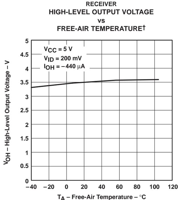
† Only the 0°C to 70°C portion of the curve applies to the SN75176B.
