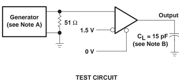
NOTES: A. The input pulse is supplied by a generator having the following characteristics: PRR  $\leq$  1 MHz, 50% duty cycle,  $t_r \leq 6$  ns,  $t_f \leq 6$  ns,  $Z_O = 50 \Omega$ .
