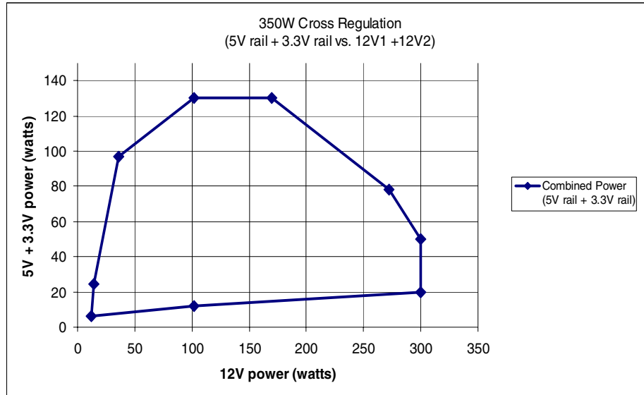
Figure 3. Cross Loading Graph for 350W Configuration
