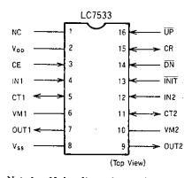
Note 1: No bonding exists on the inside of NC pin. It is recommended that the outside should be shorted to  $V_{DD}$ ,  $V_{SS}$ , etc. on the printed circuit board.
