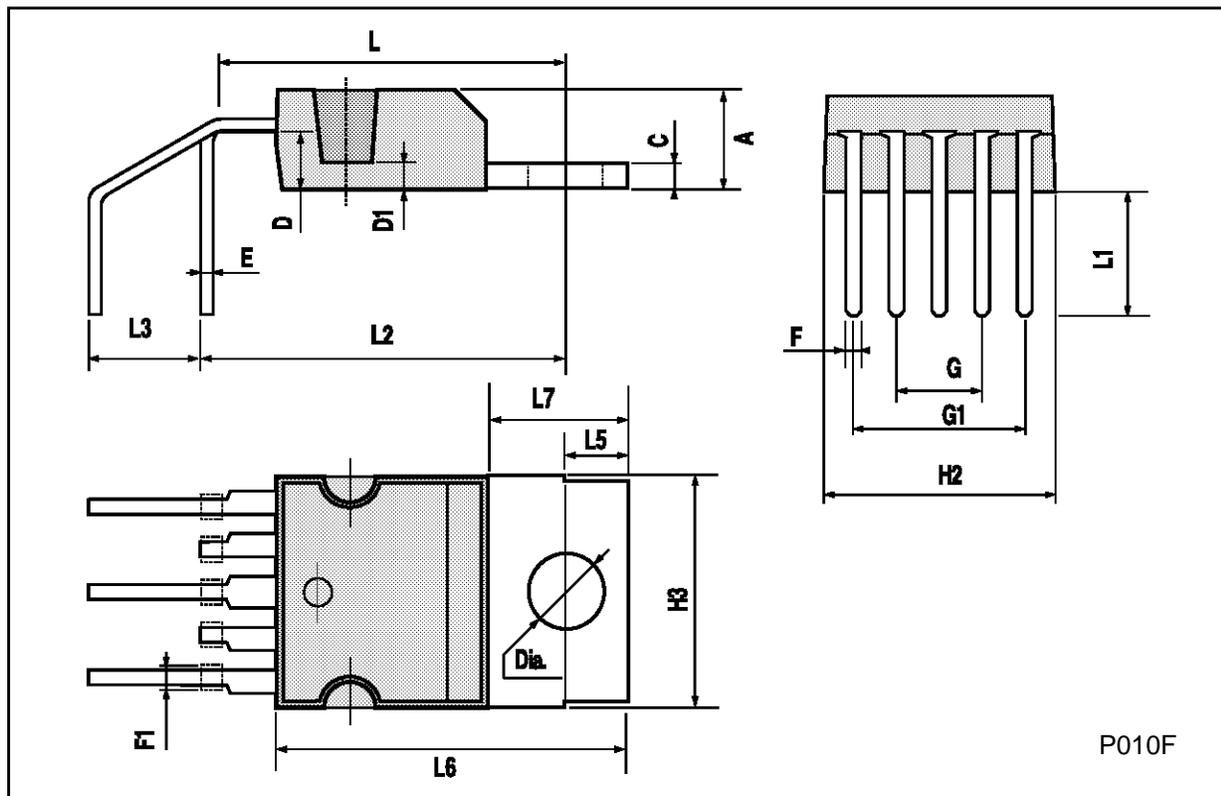
**Pentawatt (In-Line) MECHANICAL DATA**
