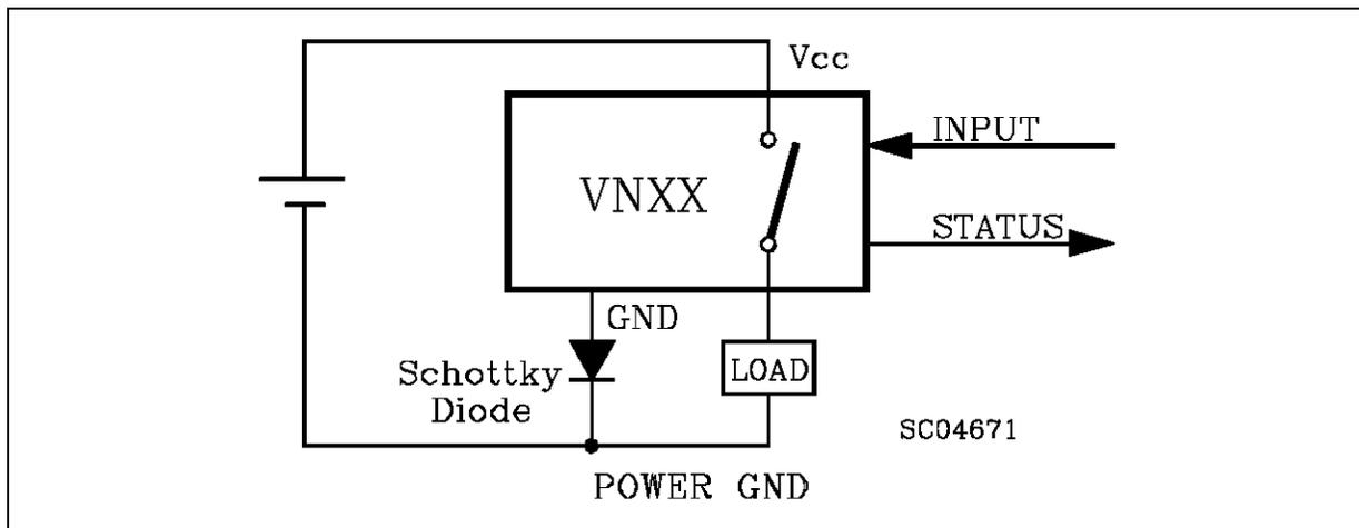
**Figure 4:** Typical Application Circuit With Separate Signal Ground
