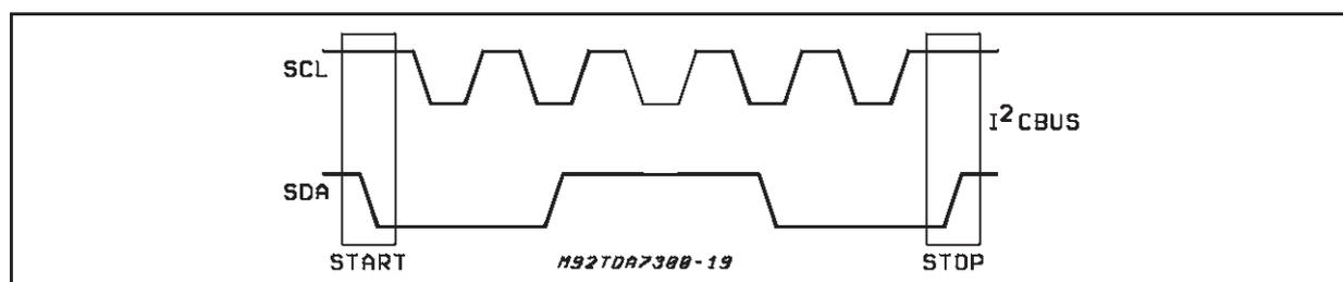
Figure 5: Acknowledge on the I<sup>2</sup>C BUS
