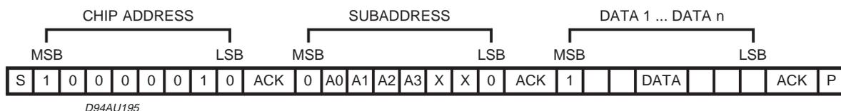
2) one subaddress, (with incremental bus) , with n data (data1 that concerns subaddress+1, data 2 that concerns subaddress+ 2 etc.)
