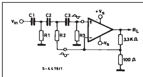
The proposed circuit can realize combined power amplifiers and 12dB/octave or 18dB/octave high-pass or low-pass filters.
