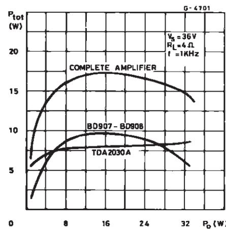
Figure 12 : Single Supply High Power Amplifier (TDA2030A + BD907/BD908)
