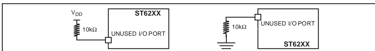
Figure 62. Two typical Applications with unused I/O Pin
