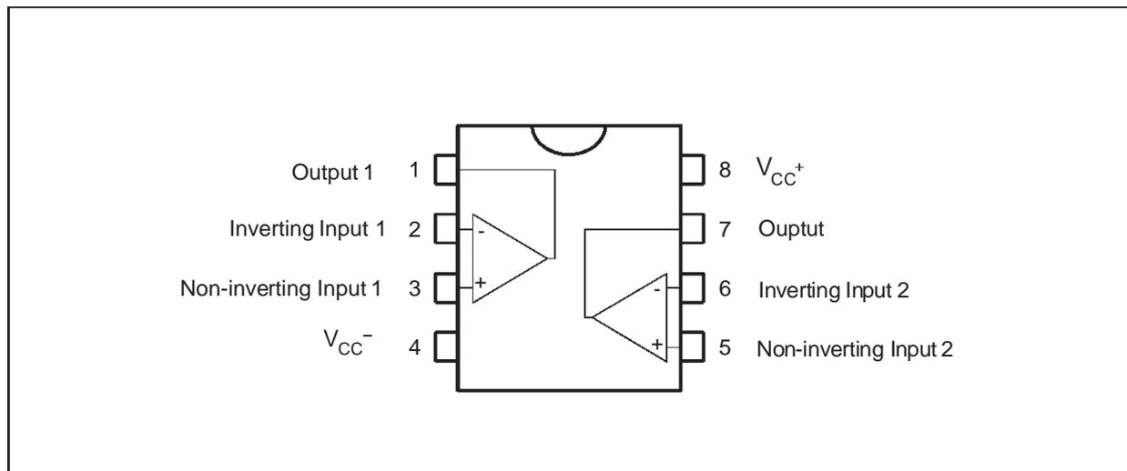
**SCHEMATIC DIAGRAM** (for 1/2 MC33172)
