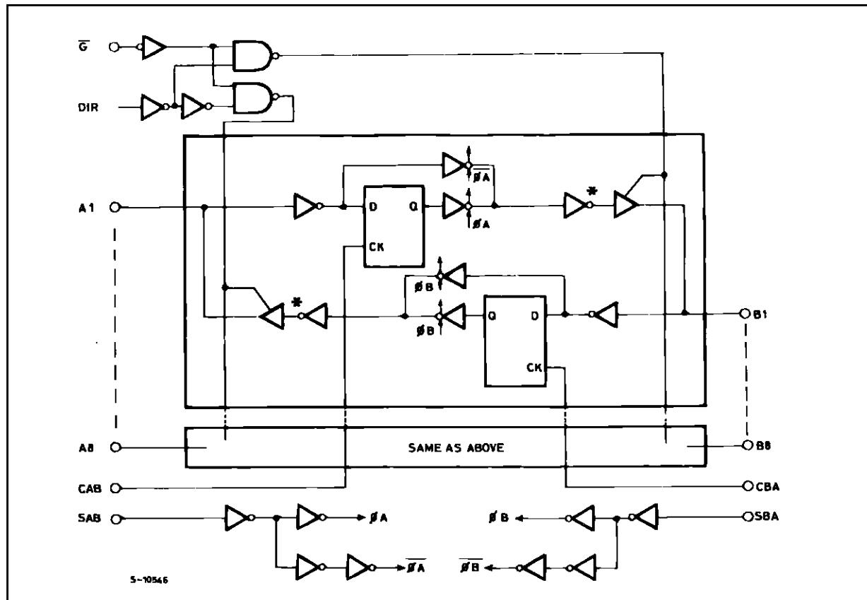
Note : In case of M54/74HCT646 output inverter marked \* at A bus and B bus are eliminated.
