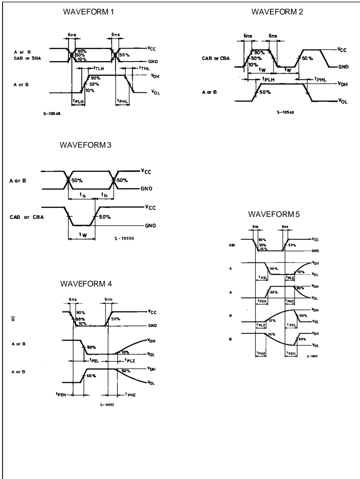
TEST WAVEFORM  $I_{cc}$  (Opr.)
