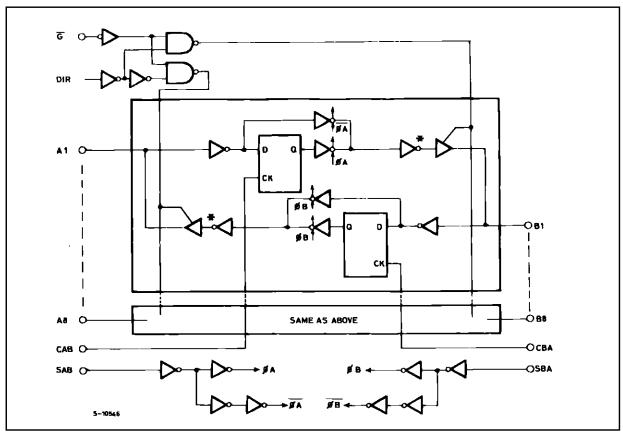
Note: In case of M54/74HC646 output inverter marked \* at A bus and B bus are eliminated.
