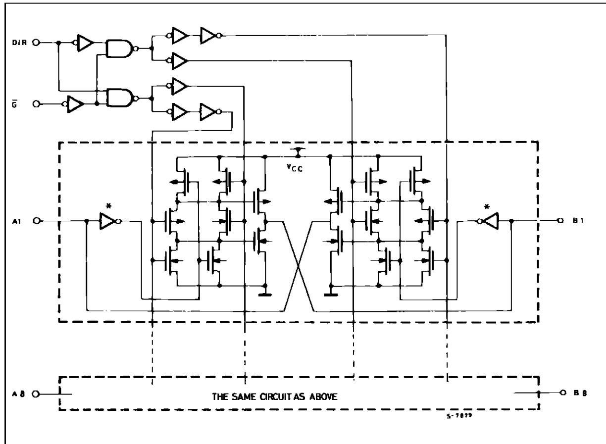
NOTE: IN CASE OF HC245 OR HC643, INPUT INVERTERS MARKED\* AT A BUS AND B BUS ARE ELIMINATED RESPECTIVELY
