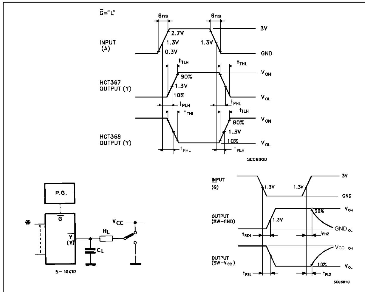
Note : Such a logic level shall be applied to each input that the output voltage stays in the opposite side to the switch connection level, when the output is enabled.
