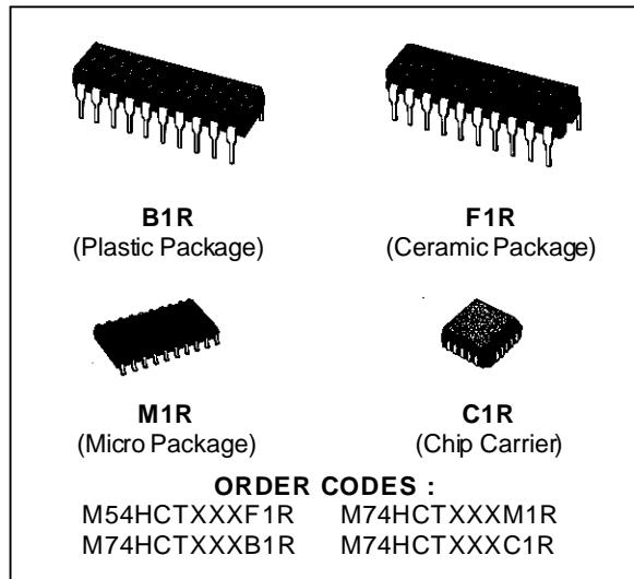
characteristics that are fully compatible with 54/74 LSTTL logic families. M54/74HCT devices are designed to directly interface HSC<sup>2</sup>MOS systems with TTL and NMOS components.
