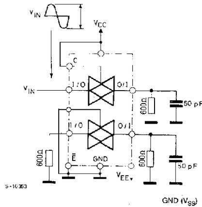
**BANDWIDTH AND FEEDTHROUGH ATTENUATION**
