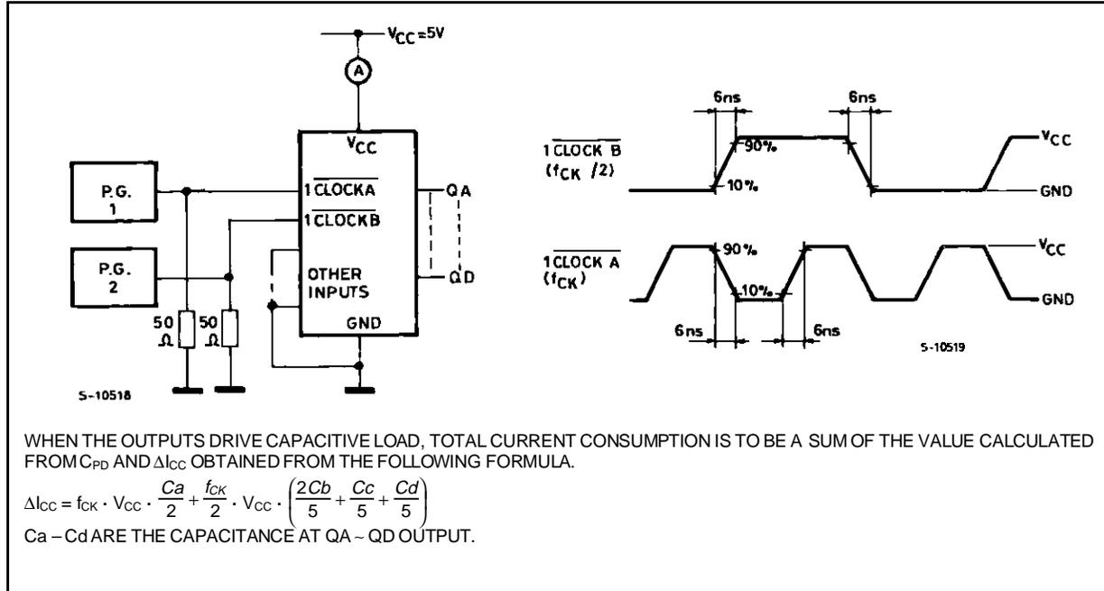
SWITCHING CHARACTERISTICS TEST WAVEFORM
