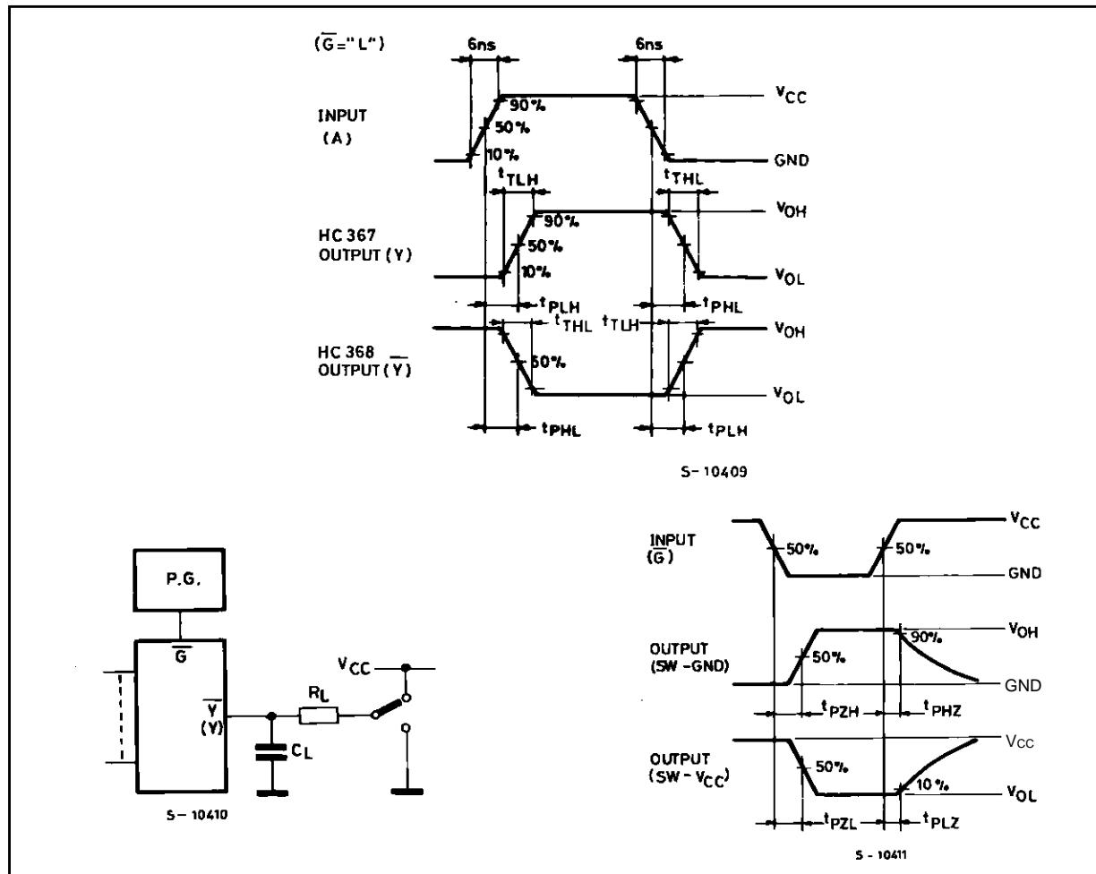
Note: Such a logic level shall be applied to each input that the output voltage stays in the opposite side to the switch connection level, when the output is enable.
