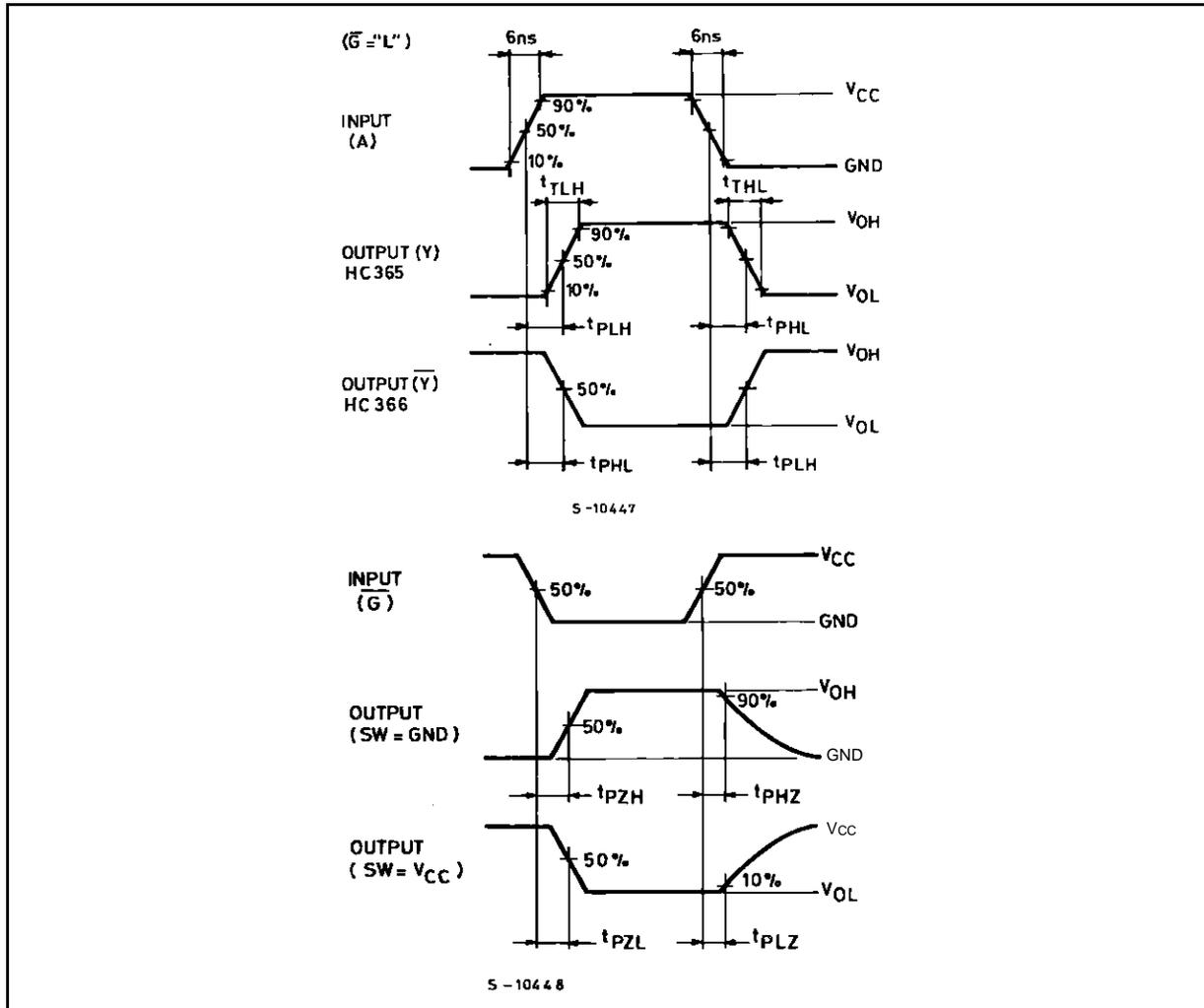
**Note :** Such a logic level shall be applied to each input that the output voltage stays in the apposte side to the switch connection level, when the output is enable.
