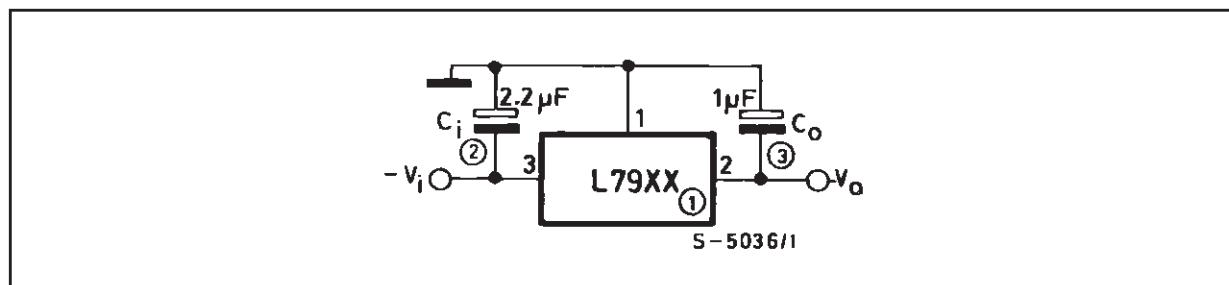
**ELECTRICAL CHARACTERISTICS FOR L7905C** (refer to the test circuits,  $T_j = 0$  to  $150^\circ\text{C}$ ,  $V_i = -10\text{V}$ ,  $I_o = 500\text{mA}$ ,  $C_i = 2.2\text{\mu F}$ ,  $C_o = 1\text{\mu F}$  unless otherwise specified)
