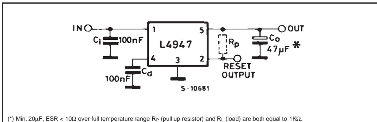
(\*) Min. 20 $\mu\text{F}$ , ESR < 10 $\Omega$  over full temperature range  $R_P$  (pull up resistor) and  $R_L$  (load) are both equal to 1K $\Omega$ .
