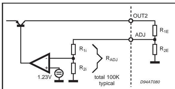
Connecting a resistor divider  $R_{1E}$ ,  $R_{2E}$  to the ADJ, OUT2 pin the output voltage 2 can be programmed to the value of
